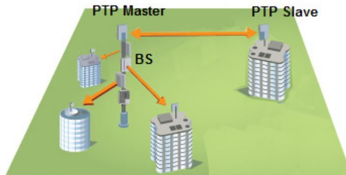
*In the above, there are two separate sites shown. Each site has multiple co-located base stations. The two sites are connected using a PTP link. This is NOT allowed because a PTP Slave unit must be located at one of the two sites and it cannot be co-located with base stations.*
