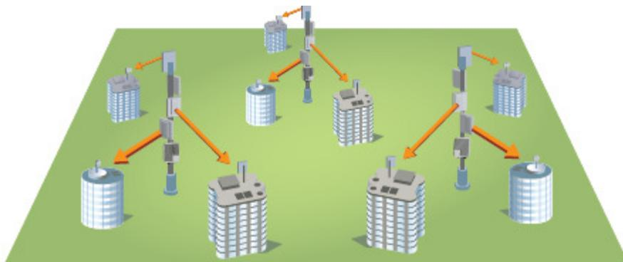
Shown here are three different sites. Each site has multiple base stations co-located. Through the use of a common GPS signal, all of these base stations can be synchronized.
