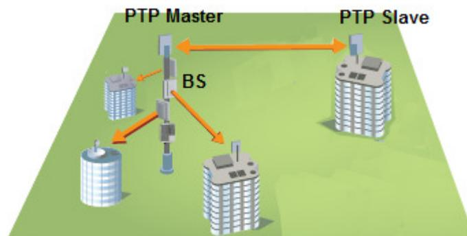
*In the above diagram, the site on the left has many base stations co-located. A PTP link is used to backhaul the base station traffic to another site (central gathering point, for example). A PTP Master unit is located at the base station site on the left and it is connected to the PTP Slave unit at the other site.*
