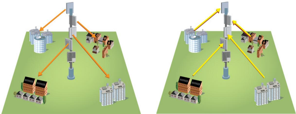
*The left diagram indicates a downlink time slot during which all base stations are transmitting and sending data to subscriber units. The right diagram indicates a time slot during which all base stations are receiving data from subscriber units.*
