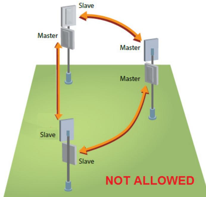
*In the above ring case with an odd number of nodes, you cannot make the co-location work at one of the sites. One site (the top site in this example) has to have a slave and a master unit, not an allowable condition for GPS synchronization.*
