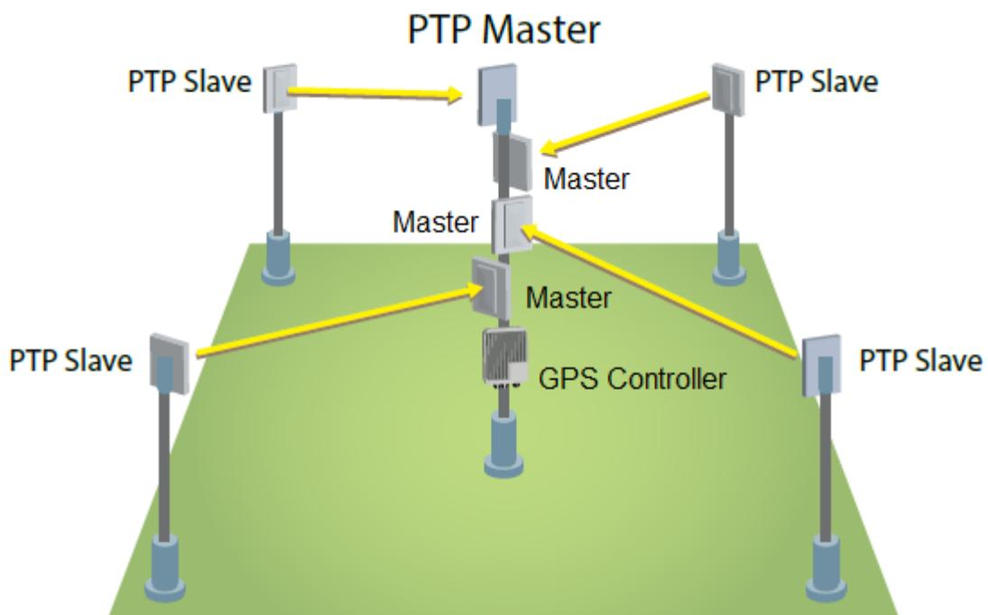
*At the central site, make sure to configure radios to be PTP Master units so that all co-located radios are transmit/receive synchronized. All of the Master PTP units need to be connected to the GPS Controller, shown at the bottom of the central site.*
