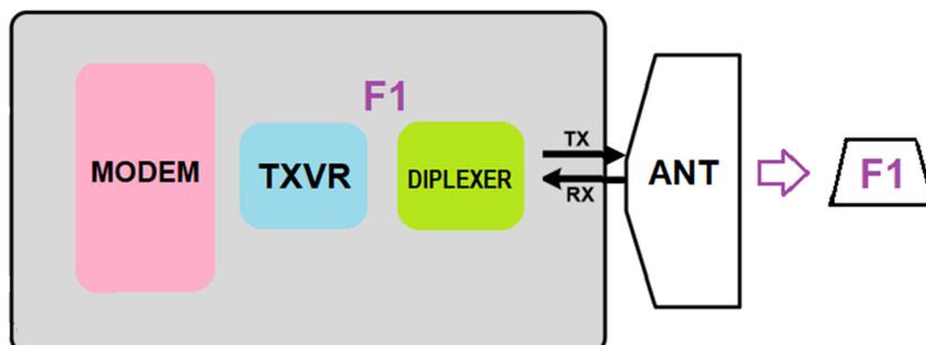
Many of the microwave links deployed today are configured in the “1+0” manner, which is basically one primary radio link + zero redundant backup path.
