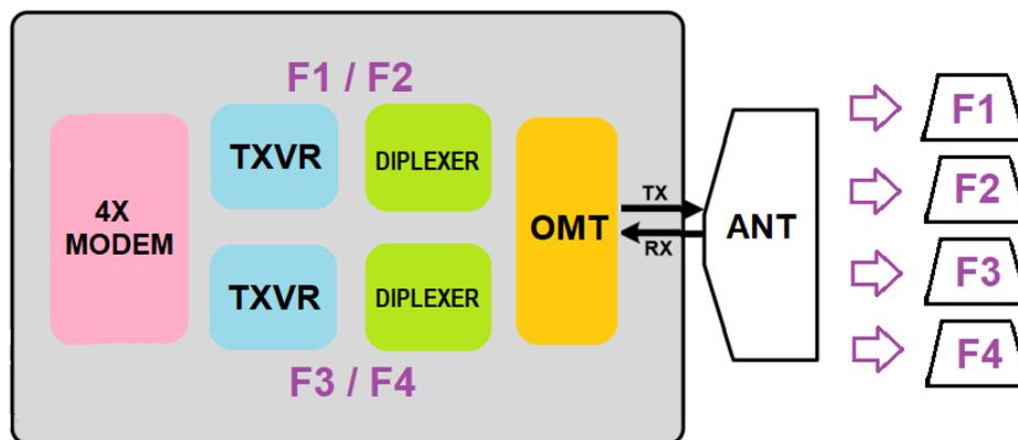
This scheme essentially incorporates the sub-channel scheme just discussed in a dual-transceiver radio terminal. The net effect is that a single terminal carries four independent signal streams, F1 to F4, similar to a standard 4+0 configuration, except that in this case, all of the data is carried by a single radio terminal with a single-polarization antenna. (same restrictions as in the above single transceiver case, i.e. to put all 4 channels within the diplexer range, are applicable here).
