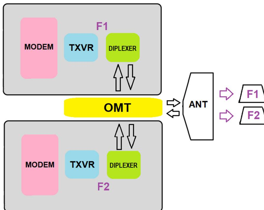
This is the traditional way of increasing capacity – use two radio units (each operating at a different channel) and combine the signal using an external OMT device. The drawback is that (a) the equipment cost is more than double (two radios + OMT) and (b) tower loading is also more than double for the same reason.
